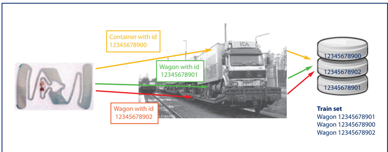
Illustration 2: RFID Tag with an individual, owner specific identification stored in the data base (leads to misinterpretation of which object has been observed)
